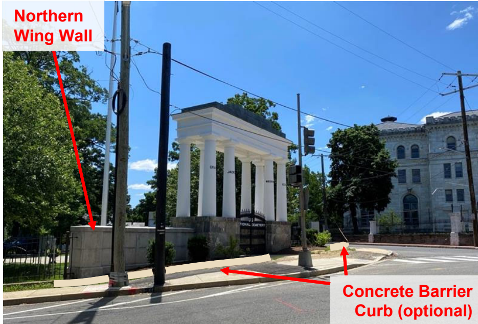
Illustration of proposed barrier concrete curb, viewed from the intersection of Rock Creek Church Rd NW and Harewood Rd NW looking southeast toward the SAHNC Main Entrance Gate northern wing wall (2024)
